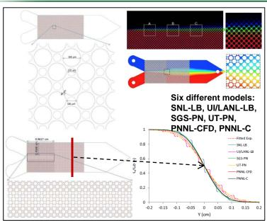
(Left) Micromodel configuration of different pore structures including post, pore-throat, and pore-body. Total four different structures were tested. (Upper right) Measured concentration image (top) and a simulated concentration distribution (bottom) (Lower right) Experimental and numerical concentration profiles along the transect.
